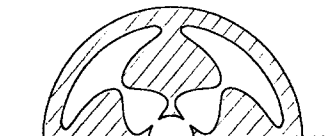
Fig. 2. Finned tube geometries which maximize Nu_e when \alpha is equal to 0.8, \beta to \pi/4 and \gamma to 500.
